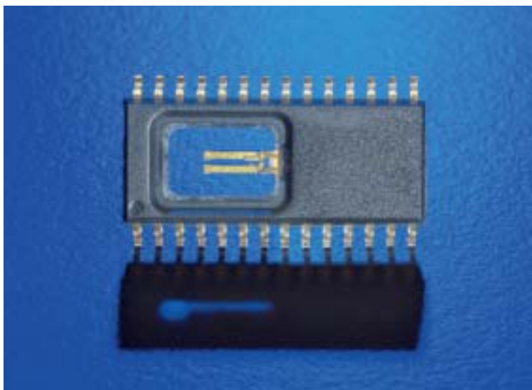
Multi-chip module tuning-fork sensor
